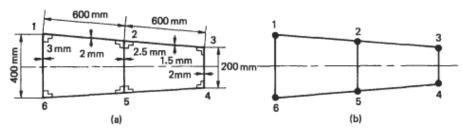
**Q.4A)** A beam having the cross section shown in Figure is subjected to a bending moment of 1500 Nm in a vertical plane. Calculate the maximum direct stress due to bending stating the point at which it acts. (07)
