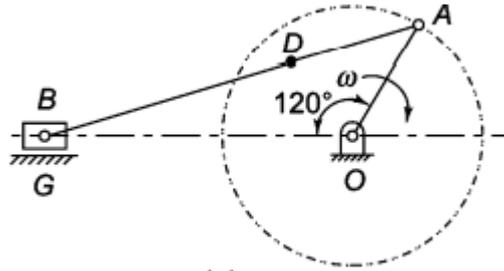
Above fig. shows configuration of an engine mechanism. The dimensions are following:
