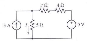
(5) Employ Norton's theorem to obtain a simple two-component equivalent of the circuit shown in figure.
