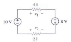
4. In the circuit of figure, find the voltage drop across 2  $\Omega$  just before t = 0.
