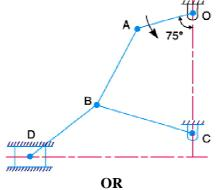
B) In a pin jointed four bar mechanism as shown below, the crank rotates uniformly at 100 r.p.m. (08) Locate all the instantaneous centres and find the angular velocity of the link BC.
